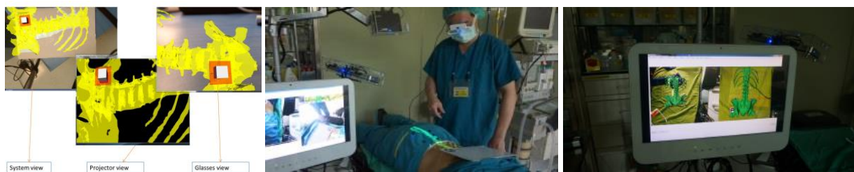
Figure 2: The mixed reality to interact with the spinal image from a real patient. The image demonstrates the proposed MR and poses tracking work in permit results. The surgeon adopts the assisted system for surgical planning, and then checks simulation steps of the vertebroplasty surgical procedure.
