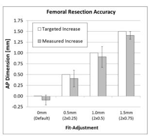
**Methods:** The accuracy of guide-positioning and bone-cutting with A.R.T. was assessed in bench testing on synthetic bones (Sawbones®) using an optical comparator.
