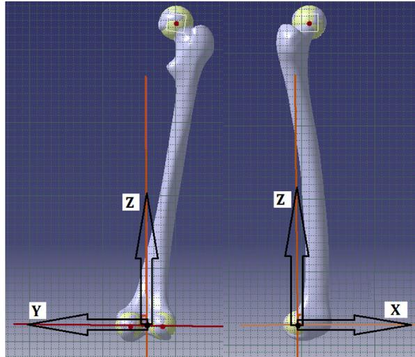
Figure 1- The proposed local coordinate system for a right femur.
