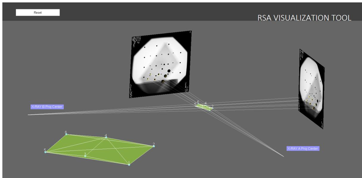
Figure 1: Screenshot of custom-made software showing reconstructed phantom markers within the RSA setup
