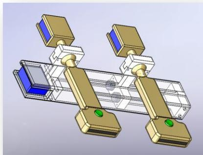
Figure 1 – The ultrasound device for the estimation of the pelvic tilt.
