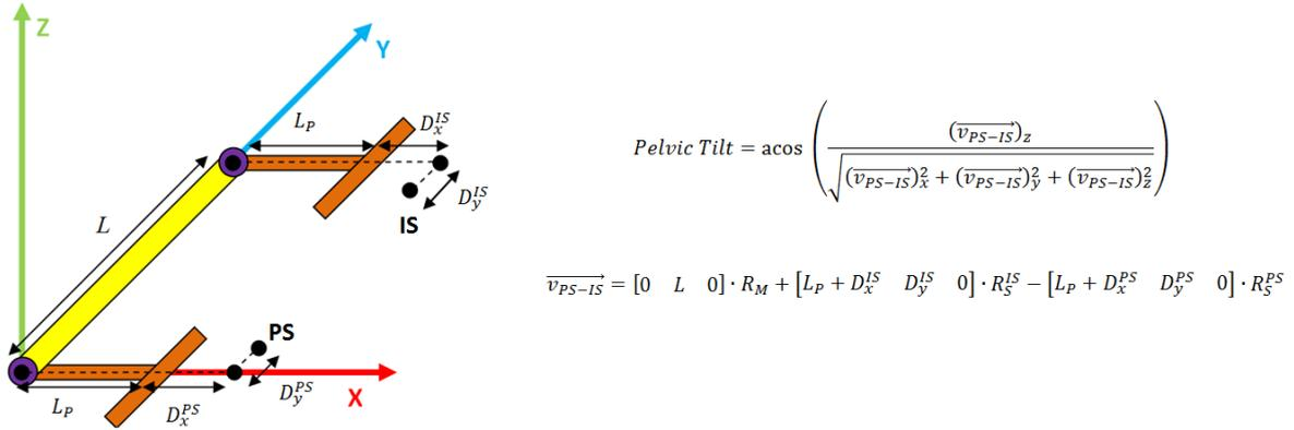
**Figure 2 – Computation of the pelvic tilt, with L the distance between the center of rotation of the probes, L<sub>P</sub> the length of the probes, D the position of the bony landmark (IS or PS) along the axis (x or y) of the US frame, R the rotation matrices (main body (M), IS probe or PS probe), given by the inertial sensors.**
