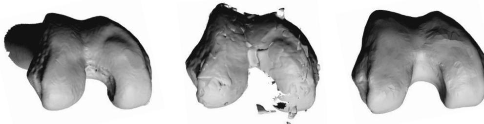
**Figure 3: CT based reconstruction of a solid foam bone phantom (*SAWBONES*) of the distal femur (left), segmentation and registration result of surface patches from ultrasound volume images (middle), reconstruction result after fitting a statistical shape model (right).**
