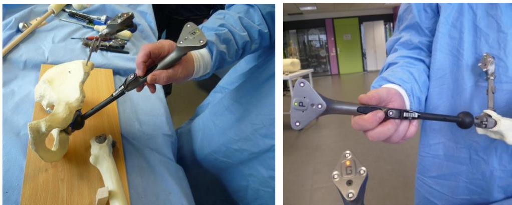
Figure 1. Illustration of the “HipBall” concept with ONE device used to digitize both the cup and the neck.
