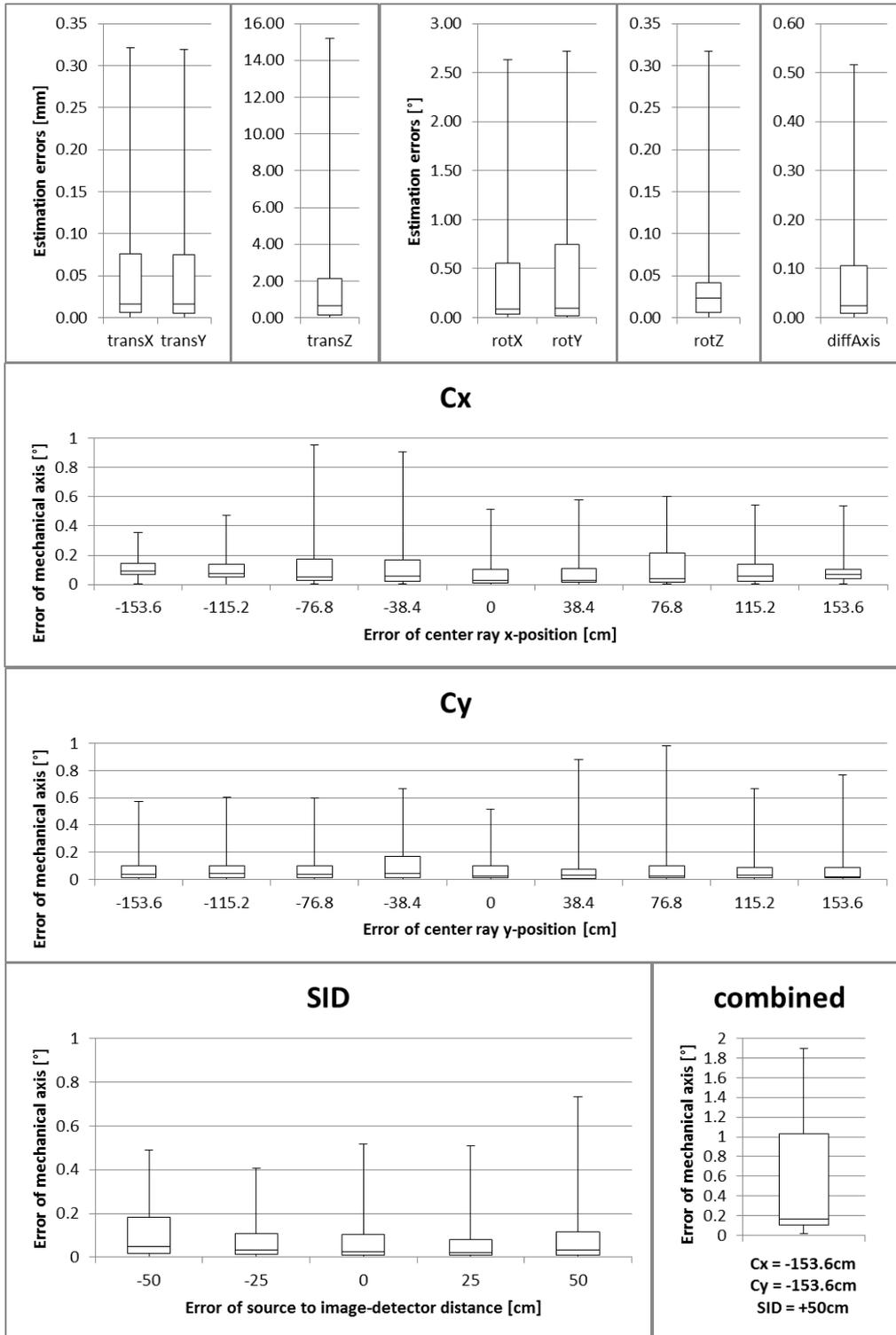
Figure 2: Accuracy of mechanical axis determination and influence of incorrect calibration data.
