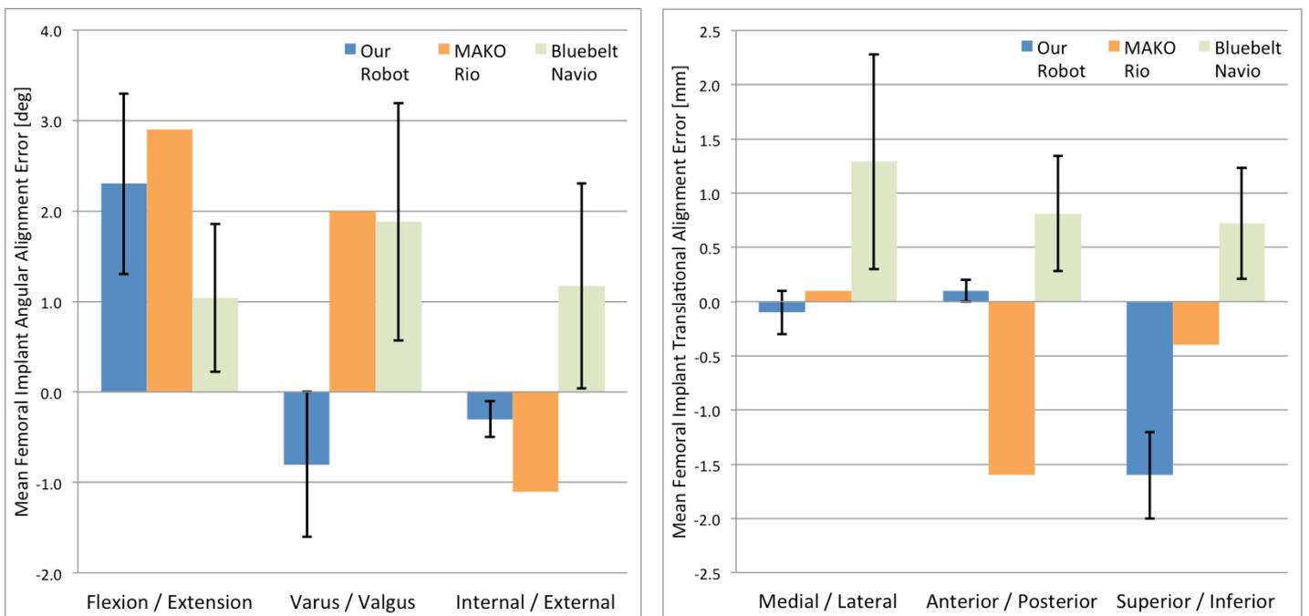
Figure 2: Comparison of three robotic systems in femoral component angular alignment error (left) and translational alignment error (right).
