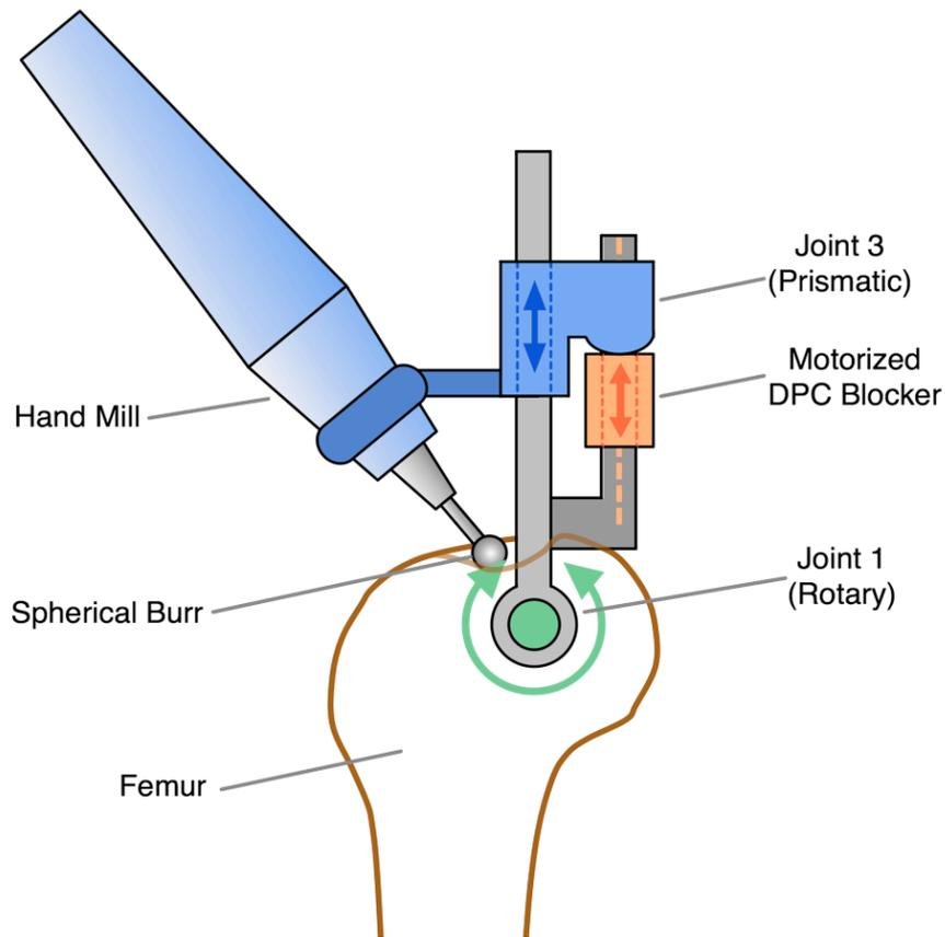
Figure 1: 2D Schematic representation of Rotary-Prismatic configuration and Dynamic Physical Constraint.
