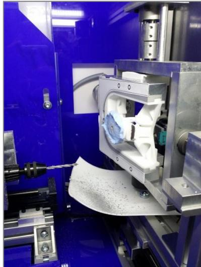
**Figure 4 - The CNC drill (fitted with sterile drill bit has been completed its modification of the sterile disposable element seen in the centre of the image. The drill and sterile disposable receptor assembly both configure themselves such that the hole drilled exactly corresponds to the pre-operative plan.**
