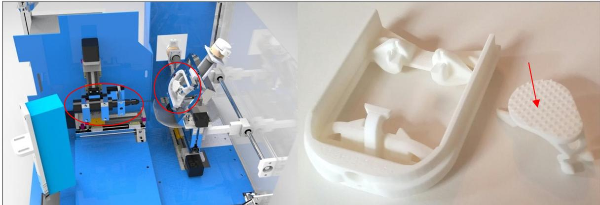
**Figure 1 – Left image: interior of the re-usable hardware element showing CNC drill and CNC receptor assembly for the sterile disposable component (red circles from left to right). Right image: Sterile disposable element (red arrow). The indicated surface has a body of mouldable material when in use. Image also shows a sterile enclosure lining allowing the sterile element to be placed into the non-sterile hardware and independently removed easily.**
