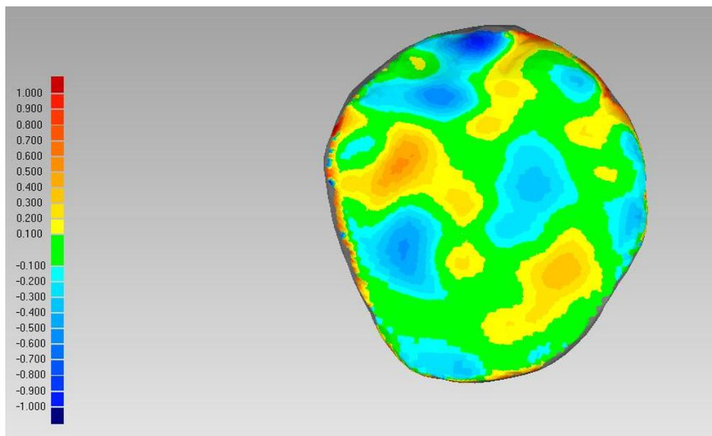
**Figure 2: Top view of the colour deviation map for the spatial distribution of the deviations between the reference (MRI) and the test (laser) model of a left tibial lateral cartilage**
